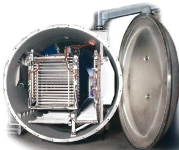
The internal vapour condenser, with built-in de-icing system, is the unique feature of all Atlas freeze dryers. The benefits: it saves space, it is more reliable, it does not cause the loss of product, and it uses less energy compared with external condenser systems.
